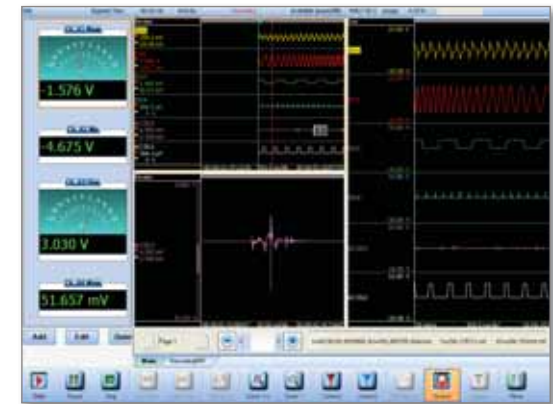
Complete test setups, including data display arrangements, are stored in and retrieved from Dimension4i using Project files.
